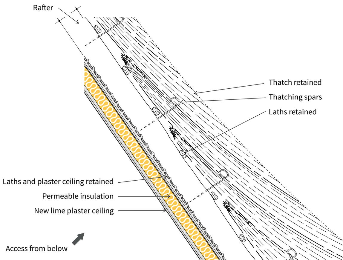
**Figure 9: Warm roof – sloping ceiling (adding insulation from below – thatch retained)**
