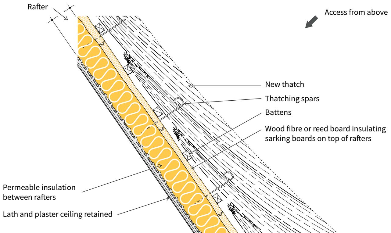
**Figure 8: Warm roof – sloping ceiling (adding insulation from above, when thatch is stripped entirely)**
