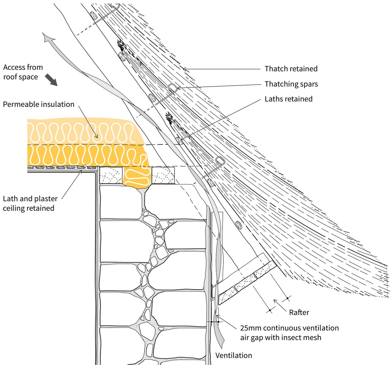
**Figure 10: Cold roof – Roof space insulation at eaves**
